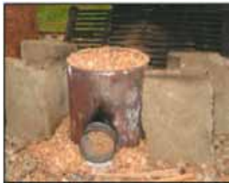
The sawdust burner made out of a 4L paint tin.
